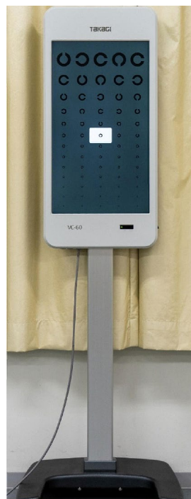
Fig. 4 Exterior of VC-60 VC60 is an optotype on an LCD display. The subjects were required to indicate the direction of the notch in the presented Landolt ring
